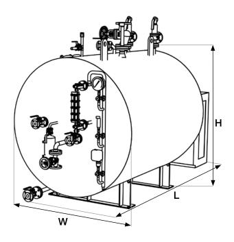
PARAT element boiler are delivered with output up to 5000 kW as standard, other sizes on request. With more than 40 years' experience with element boilers, we have developed a robust, industrial electrical boiler. PARAT element boilers are compact and have very good regulation capacity, all the way down to 15 kW.
