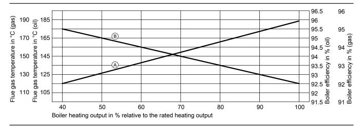
(A) Flue gas temperature in °C
